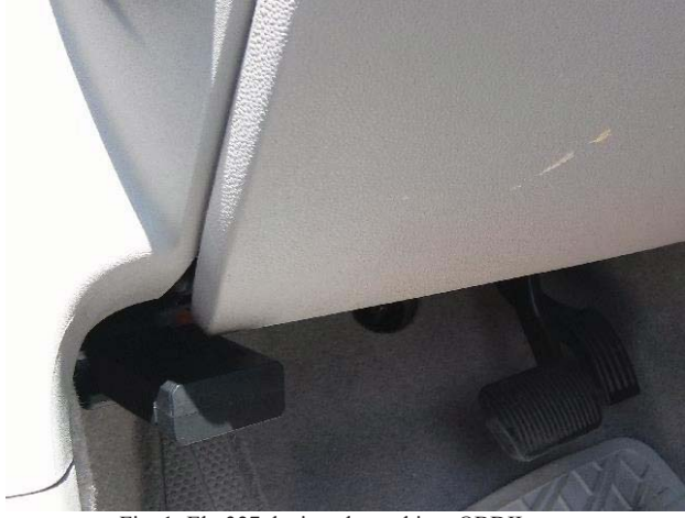
Fig. 1. Elm327 device plugged into OBDII port.
